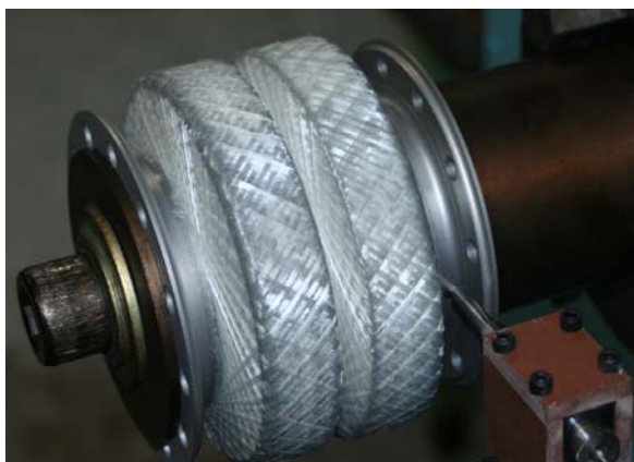
Figure 2 S2-glass flex element being wound
